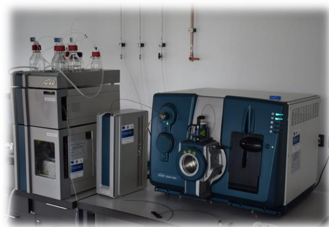
LC-MS/MS QTRAP 6500+ (AB SCIEX) at SCIENT Laboratory
